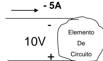
$$P = 10 \times 5 = 50W (abs) \quad P = 10 \times 5 = 50W (forn) \quad P = 10 \times (-5) = -50W (forn) = 50W (abs)$$
