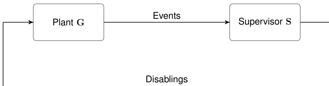
Figure 8 – Monolithic control architecture of DES in closed-loop.
